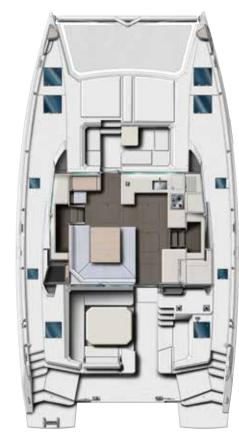
The Leopard 45 is available in either a 3 cabin, 3 head version, or a 4 cabin, 4 head version. Both layouts offer the option of additional storage, berth, or head in the forward hull.
